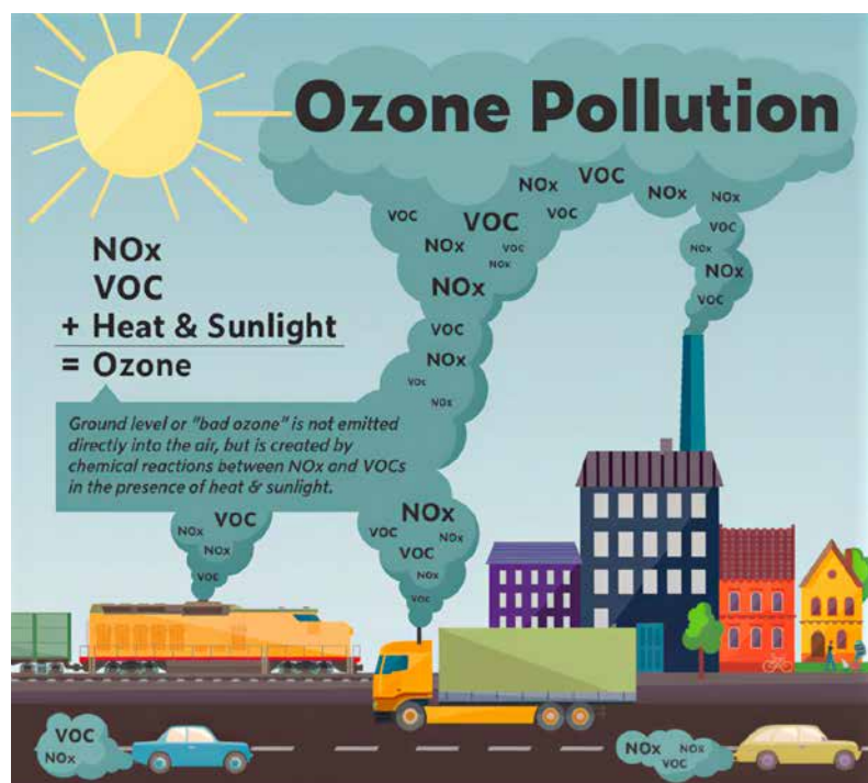
Figure 4: San Joaquin Valley Air Pollution Control District. Industrial facilities and electric utilities, motor vehicle exhaust, gasoline vapors and chemical solvents are major sources of oxides of nitrogen (NO x ) and volatile organic compounds (VOC).
